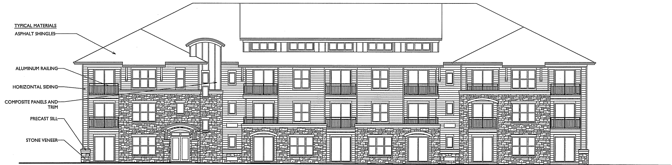
2 NORTH ELEVATION - 36-UNIT 7 SCALE: 1/8"=1'-0"
