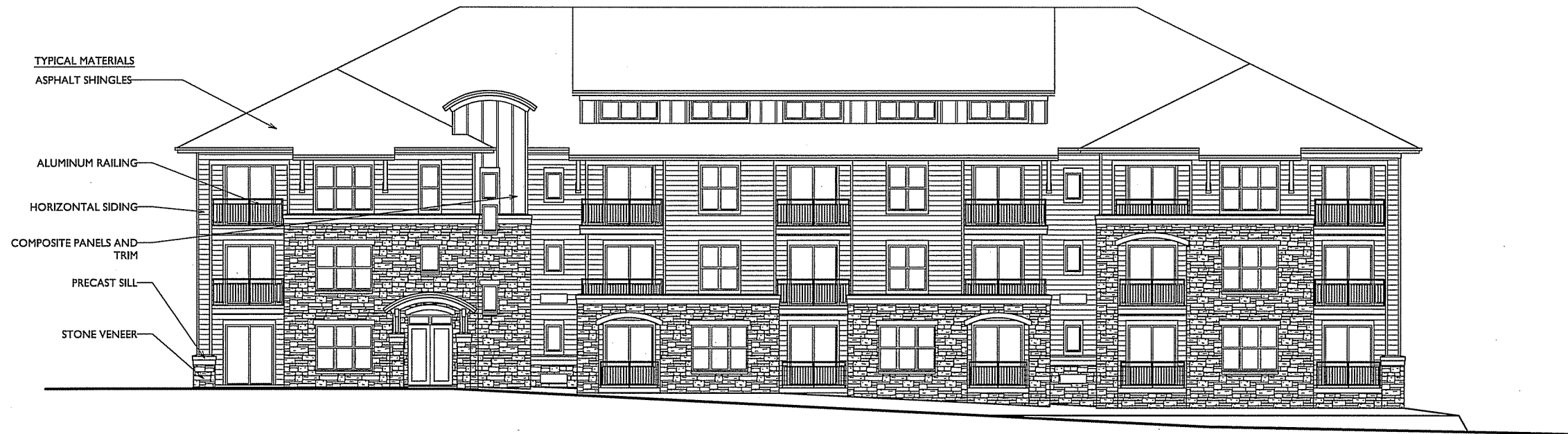
NORTH ELEVATION - 36-UNIT SCALE: 1/8"=1'-0"
