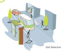
A specific inductive loop is inserted under the surface of the road. Each time a bicycle goes over the loop, the system detects the two wheels' electromagnetic signature and registers a count.
