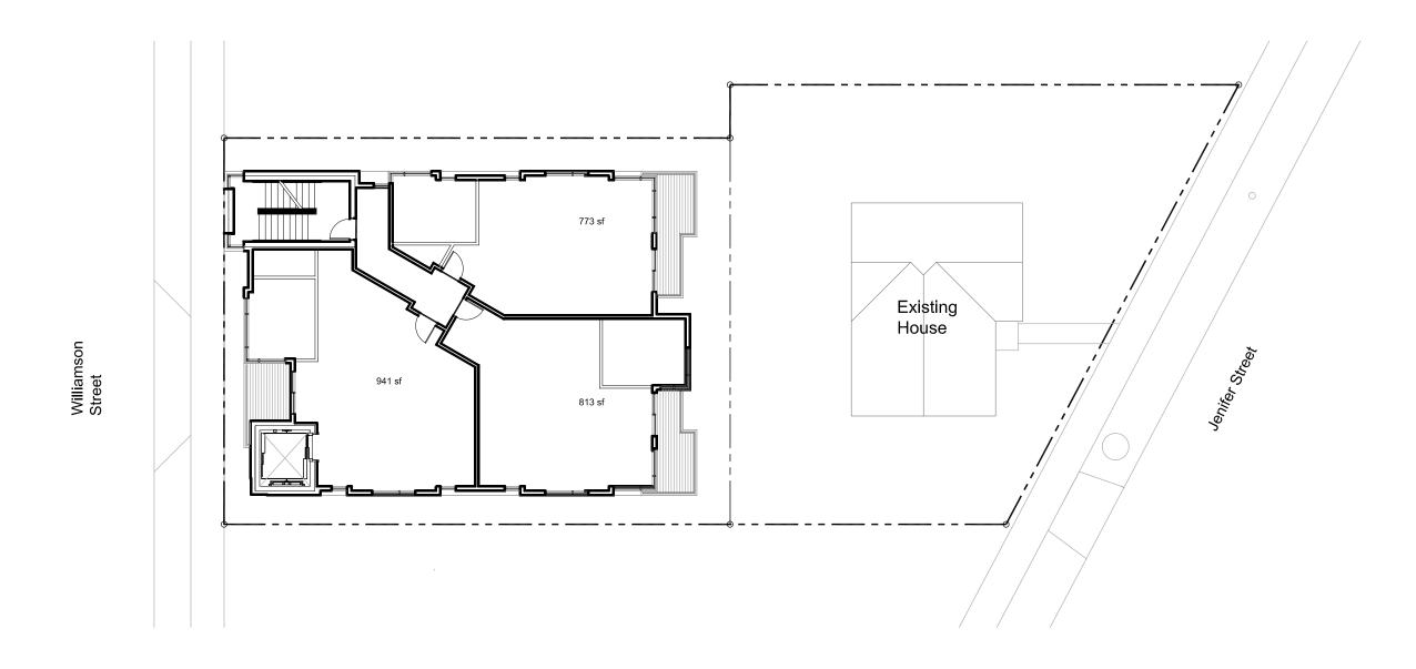
Proposed 1st Floor Plan
