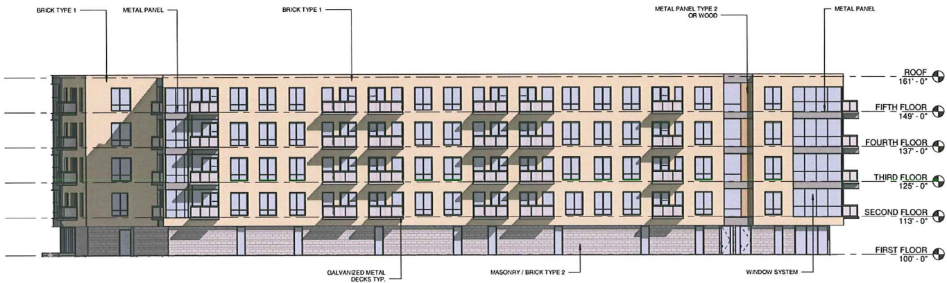
2 OVERALL WEST ELEVATION A201 1/16" = 1'-0"
