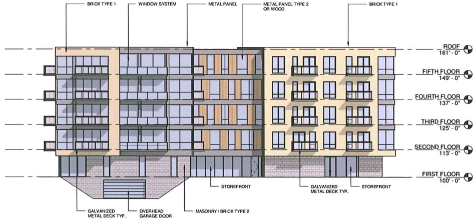
3 OVERALL SOUTH ELEVATION A201 1/16" = 1'-0"
