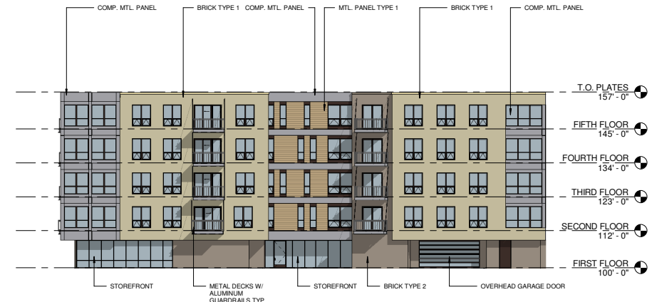
1 OVERALL NORTH ELEVATION - WEST WILSON STREET A201 1/16" = 1'-0"
