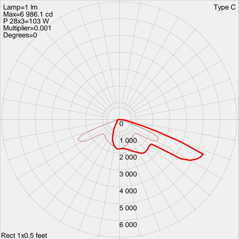
Manufacturer: COOPER LIGHTING - McGRAW-EDISON Luminaire catalog: GLEON-AA-02-LED-E1-SL4 Luminaire: GALLEON LED AREA LUMINAIRE
