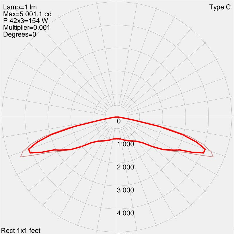
Manufacturer: COOPER LIGHTING - McGRAW-EDISON Luminaire catalog: GLEON-AA-03-LED-E1-5WQ Luminaire: GALLEON LED AREA LUMINAIRE
