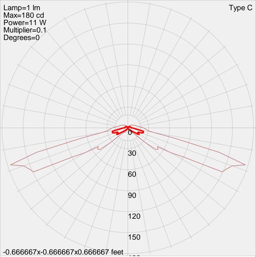
Manufacturer: KIM LIGHTING Luminaire catalog: VRB1-10LED-3500K-WH Luminaire: VANDAL RESISTANT ROUND BOLLARD LED Lamp: 10 LEDS. 3500K LUMELIDS BY PHILIPS
