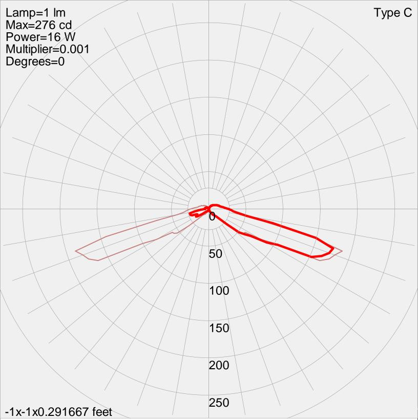
Manufacturer: KIM LIGHTING Luminaire catalog: VRB1-15LED-3500K Luminaire: VANDAL RESISTANT ROUND BOLLARD LED Lamp: 15 LEDS. 3500K LUMELIDS BY PHILIPS
