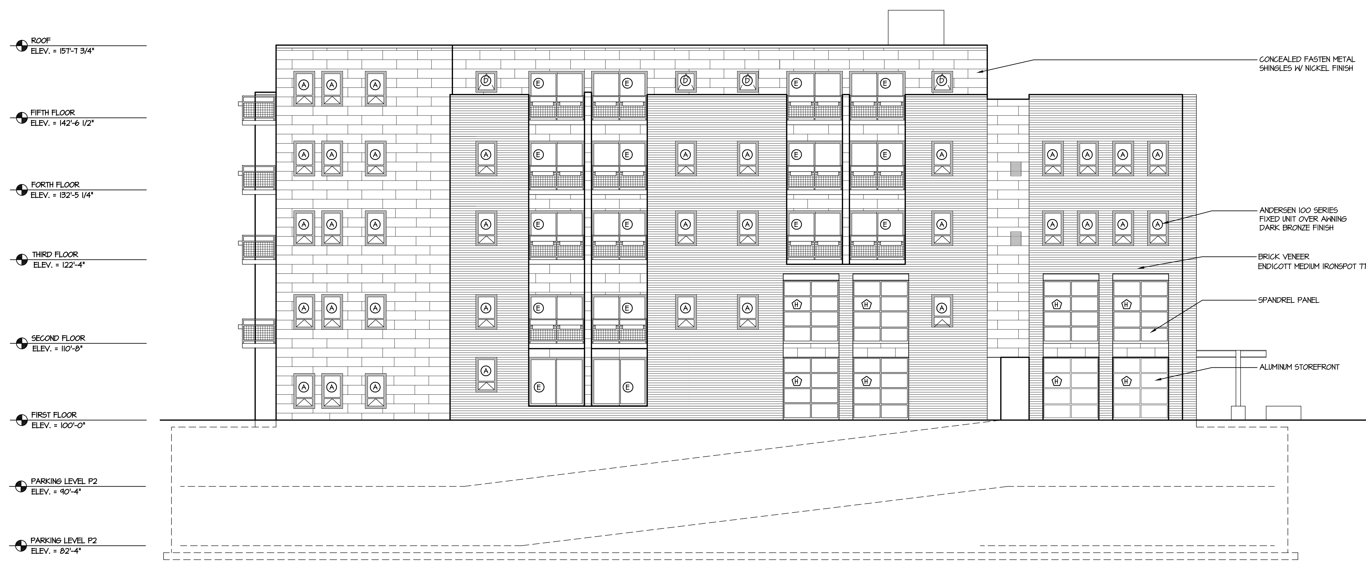
2 A2.1 NORTHEAST ELEVATION SCALE 1/8" = 1'-0"
