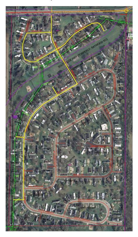
Green: Center line of existing sanitary sewer easement (Doc. 1759625) Yellow: Location of new sanitary sewer access easement
