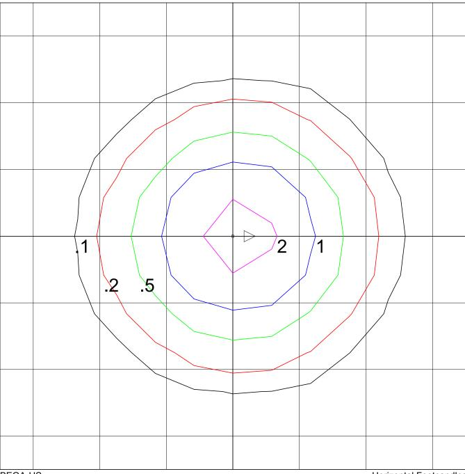
BEGA-US 3576P FULLY SHIELDED WALL MOUNTED LUMINAIRE. TEXTURED SAFETY GLASS. (1) 18W CF TRIPLE-4P Horizontal Footcandles
