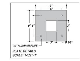
Centroid Height: 1.700 ft Sign Area: 29.500 sq ft Number of Support Columns: 3 Steel type: new Wind Pressure: 30.000 lbs/ sq ft Section Modulus: 0.216 per column 3.000 inch Steel SQUARE Tube: ( .25 inch wall),each column
