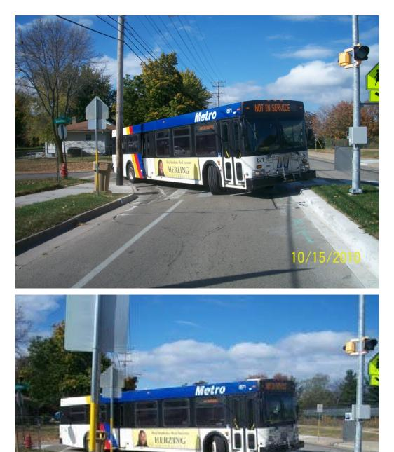
Even with an adequate "set up" for the turn, the front bumper of the bus still sweeps out over the center island. There have been occasions when buses have backed up in the intersection to avoid either the utility pole in the S.E. corner, or the light pole mounted in the island.
