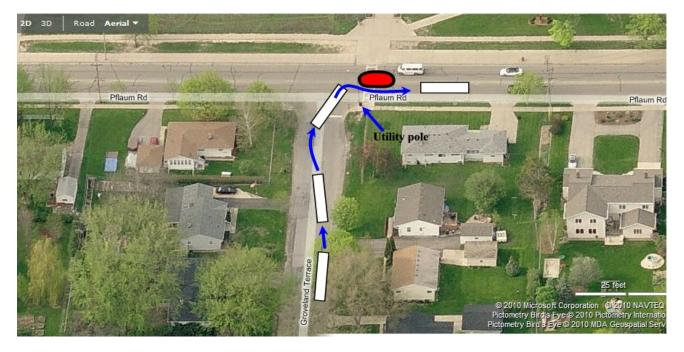
Buses need to use all of the northbound lane of Groveland Terrace plus at least half of the southbound lane in order to set up for the turn, clear the utility pole on the S.E. corner of the intersection, while simultaneously minimizing the amount of encroachment of the front bumper over the center island on Pflaum Road.
