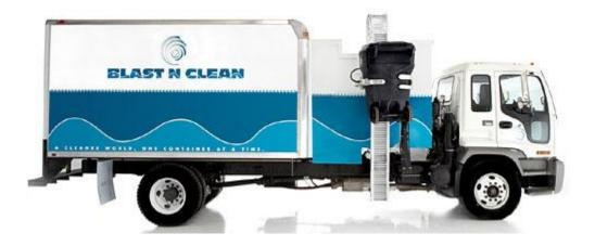
**The Commercial Truck** operates in a similar way except the truck will pick up the dumpster from the front of the truck and lift the container over the cab and hopper. Total cleaning cycle time is two minutes for these larger units.
