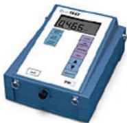
**TSI Dusttrak Aerosol Monitor** provides real time concentrations for particles in size ranges of 1.0, 2.5, 4.0 and 10.0 microns in milligrams per cubic meter. This instrument can be used to assess community airborne particulate levels in relation to USEPA particulate matter ambient air quality standards. An environmental enclosure is available to enable the user to sample outdoors for periods as long as 24 hours. The USEPA National Ambient Air Quality Standards for particulate matter are:
