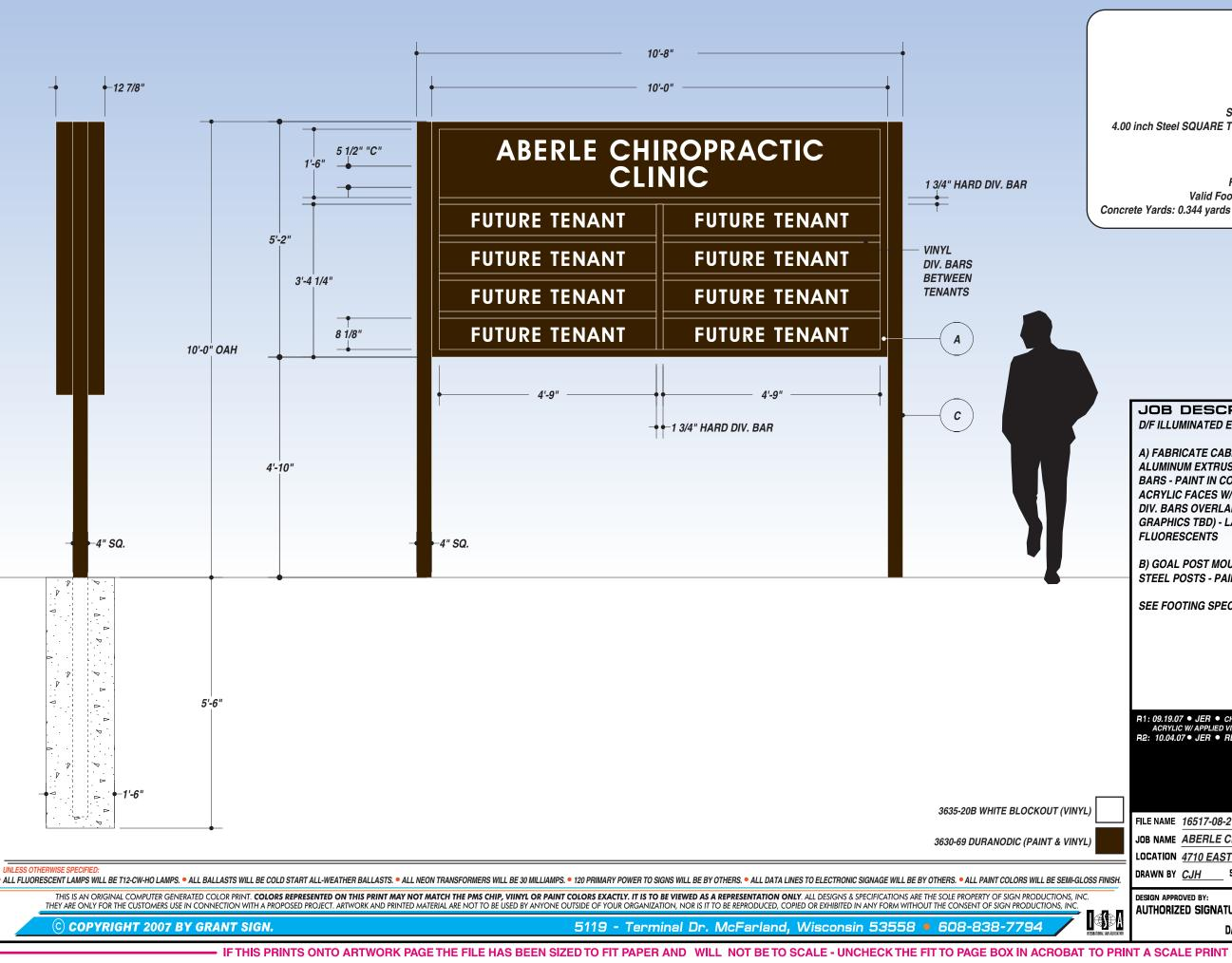
Centroid Height: 7.000 ft Sign Area: 55.000 sq ft Number of Support Columns: 2 Steel type: new Wind Pressure: 30.000 lbs/ sq ft
