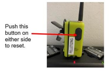
Simultaneously press the side buttons on the SC500 units.
