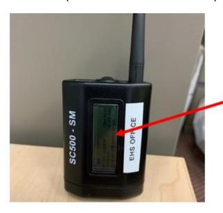
Area the TPass is assigned to shows up on screen when alarm occurs.
