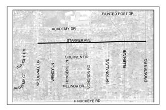
Water Main: The City will replace the existing water main along Starker Avenue (existing main Woodvale Drive to Vondron Road: 6-inch, cast iron, 1964; existing main Vondron Road to Ellen Avenue: 6-Inch, cast iron, 1956; existing main Ellen Avenue to Droster Road: 6-inch, ductile iron, 1971).
