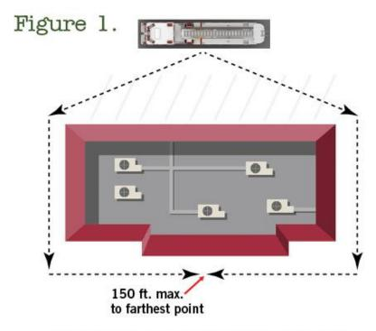
If the distance measured from the fire engine to the farthest point on the building exceeds 150 ft., additional access (fire lanes) is required.
