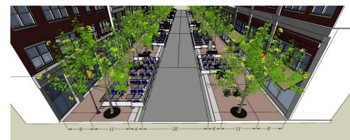
Idea 2: All pedestrians and bikes in street Ramping of some type needed – difficult due to drainage, structural slab, tripping hazards
