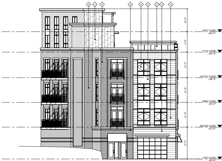
2 ELEVATION - WEST A2.1 1/8" = 1'-0"
