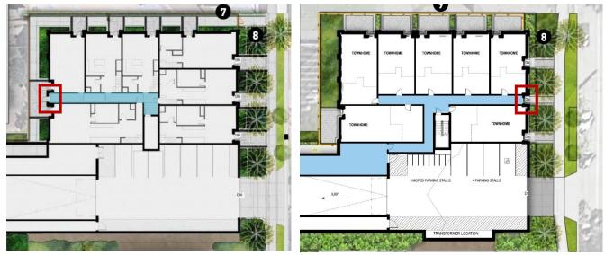
Image 1: Ground floor layout of the building's 6-story mass. <u>Left</u>: Original proposal with an exterior walkway leading to individual townhouse entrances; and Right: Revised proposal with the walkway removed and replaced with private patios
