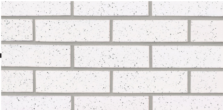
Glen-Gery "Oyster White w/ Speck" Modular brick ( 3-5/8" deep, 2-1/4" tall, 7-5/8" wide) 3/8" mortar joint, stacked bond or soldier stacked bond, additional patterns with recessed coursing
