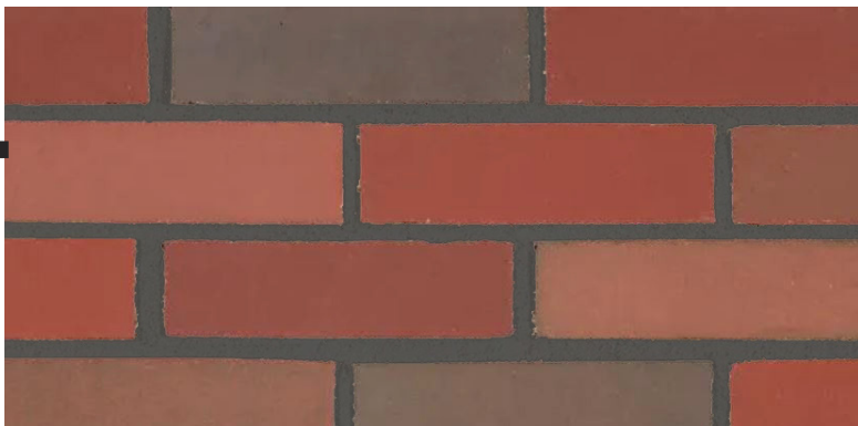
Belden Brick Co. "Colony Blend" Modular brick ( 3-5/8" deep, 2-1/4" tall, 7-5/8" wide) 3/8" mortar joint, stacked bond or soldier stacked bond, additional patterns with recessed coursing
