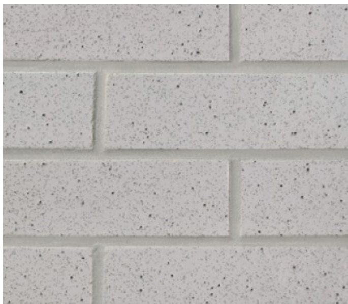
Glen-Gery "Light Grey w/ Speck" Modular brick (3-5/8" deep, 2-1/4" tall, 7-5/8" wide) comments: 3/8" mortar joint, stacked bond, soldier stacked bond, additional patterns with recessed coursing
