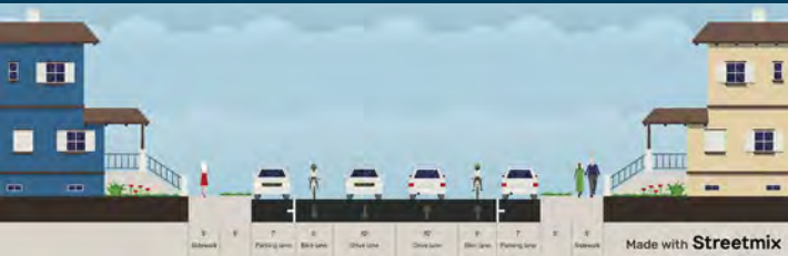
Concept with wider terraces, on-street bike lanes and single lane of parking.
