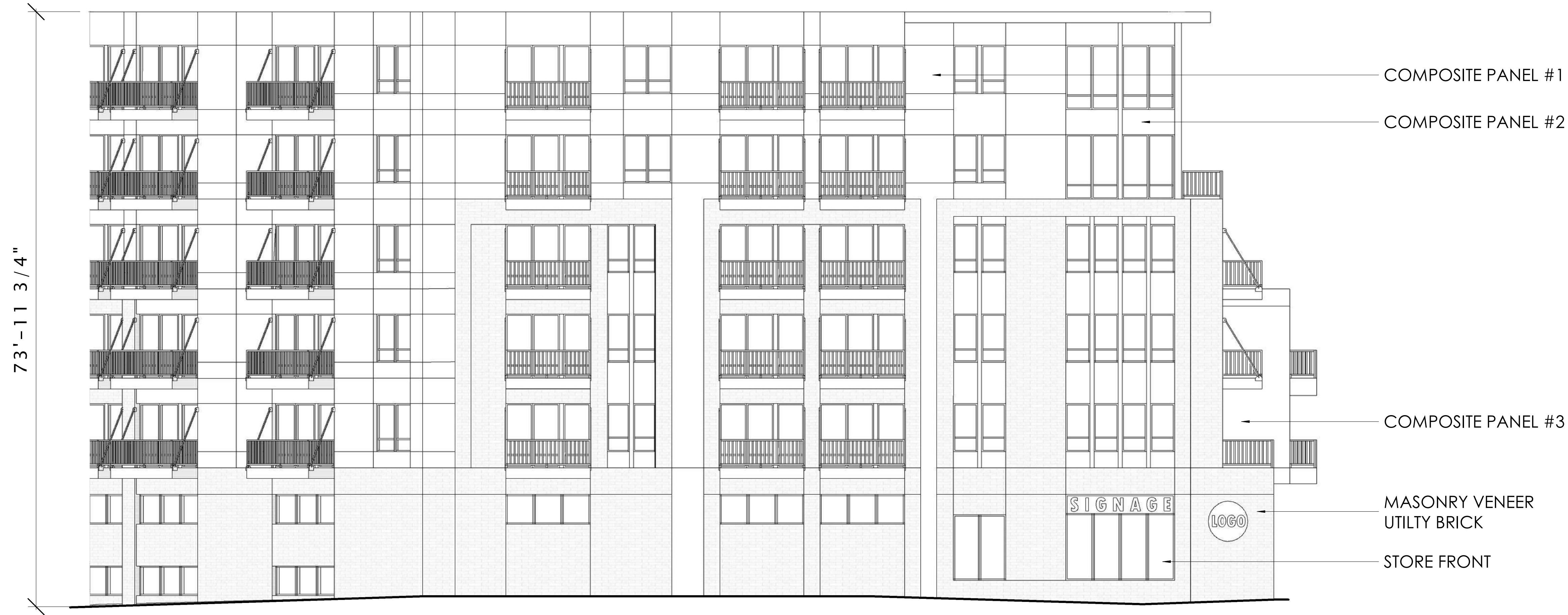
② SOUTH ELEVATION B&W 1/8" = 1'-0"
