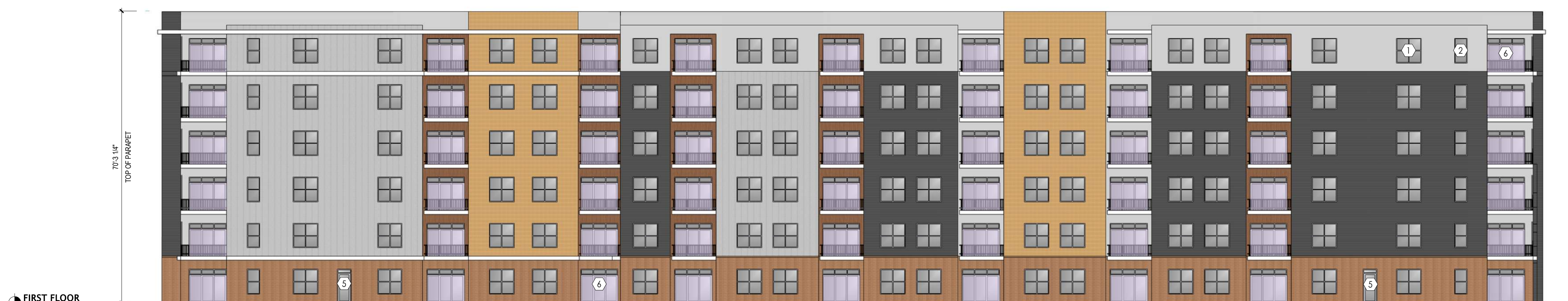
④ SOUTH ELEVATION BIRD GLASS 1/16" = 1'-0"
