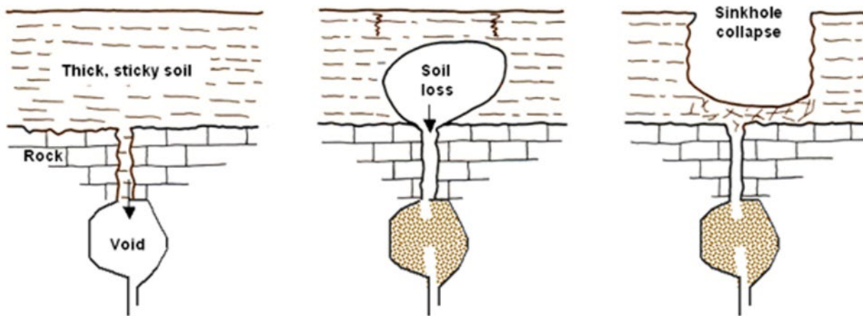
Figure 4.9.3 Sinkhole Formation Illustration
