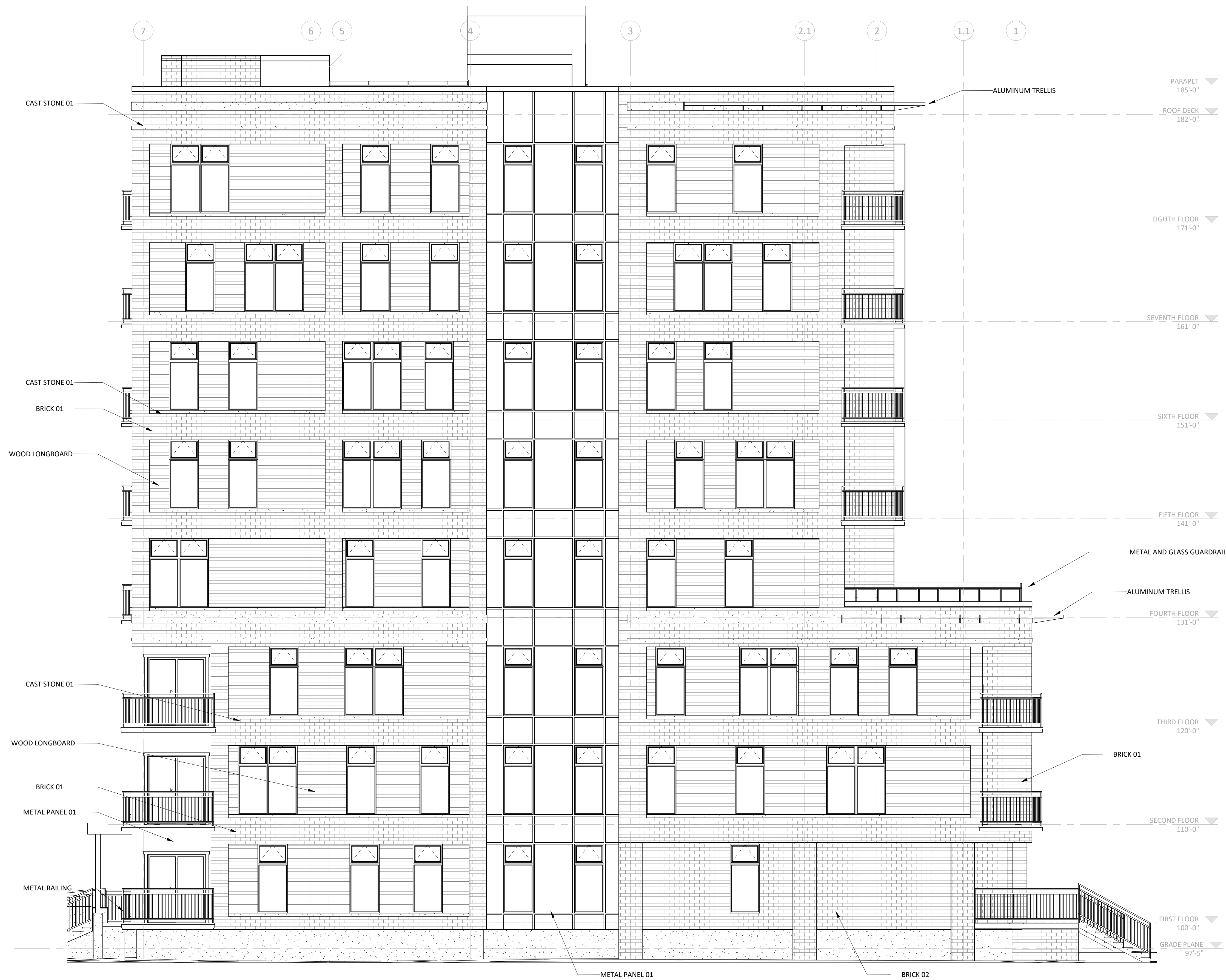
1 ELEVATION - SOUTH A-2.6 3/16" = 1'-0"
