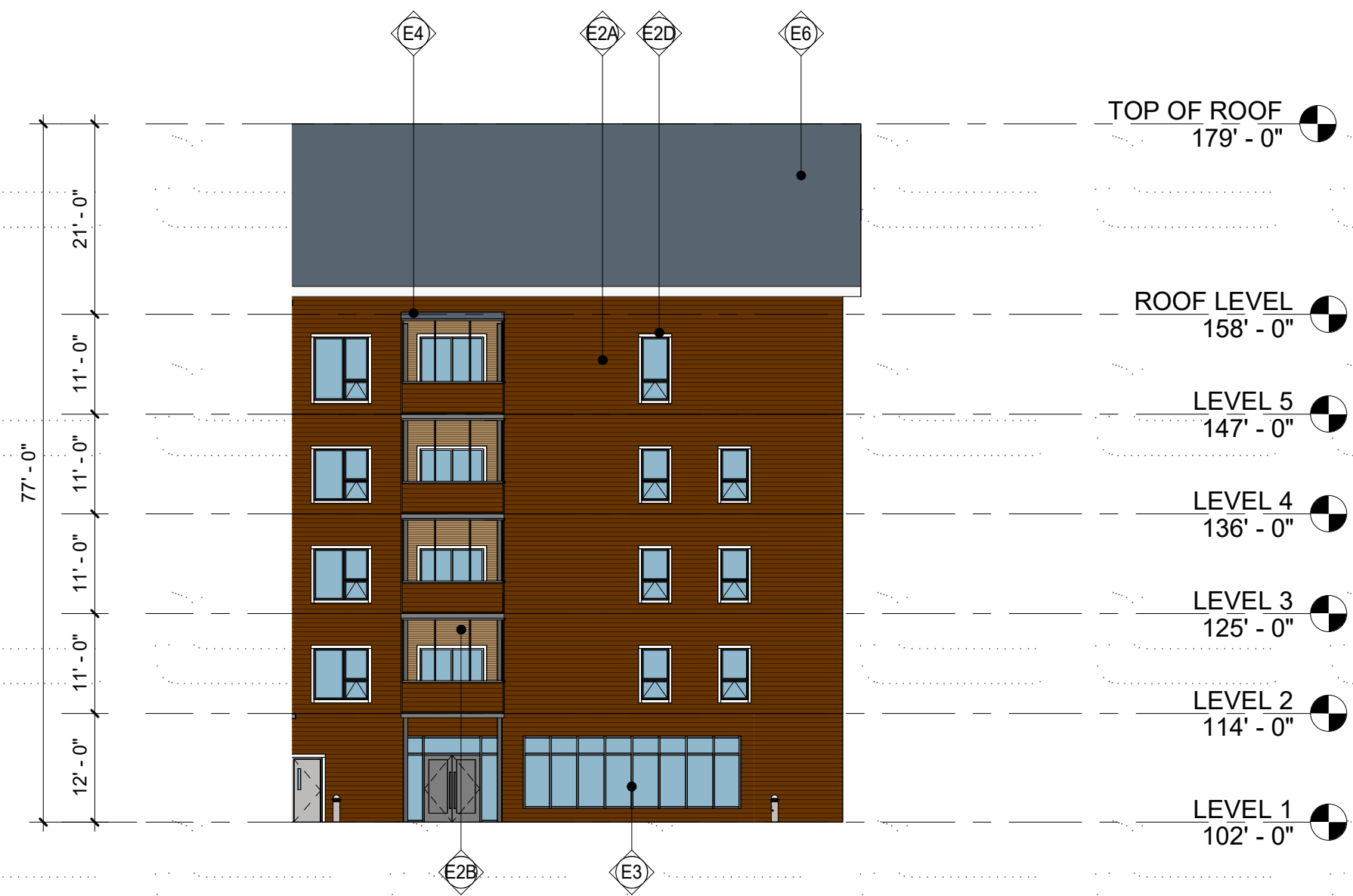
4 NORTH COURTYARD ELEVATION A3.2 1/16" = 1'-0"
