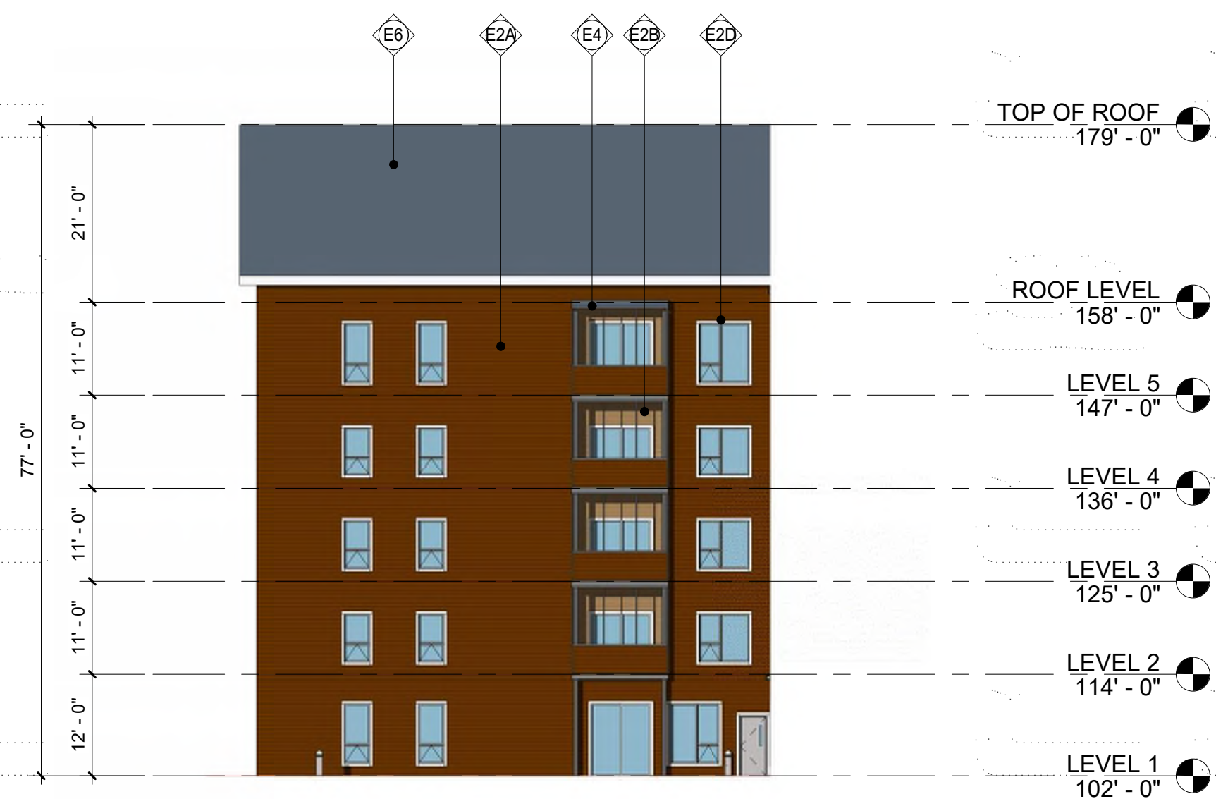
3 SOUTH COURTYARD ELEVATION A3.2 1/16" = 1'-0"
