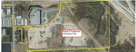
Construction of Tradesmen Drive and Kipp Street from Marsh Road east to match existing on Kipp Street including: public utility installation and street and sidewalk construction to serve all lots within the plat, bike path construction east off Kipp Street in a 22' wide easement for public pedestrian/bike purposes in proposed Outlot 2 of Replat of Tradesmen Commerce Park.
