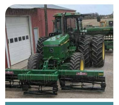
This front-mounted roller crimper allows for simultaneous flattening of a cover crop while planting a new cash crop.
