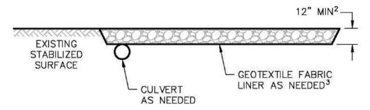
Note 1 Use hard, durable, angular stone or recycled concrete meeting the gradation in Table 1. Where this gradation is not available, meet the gradation in Wisconsin Department of Transportation (DOT) 2018 Standard Specification, Section 312, Select Crushed Material.
