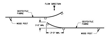
JOINING TWO LENGTHS OF SILT FENCE  $^{\scriptsize \textcircled{9}}$
