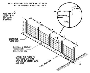
\* NOTE: 8'-0" POST SPACING ALLOWED IF A WOVEN GEOTEXTILE FABRIC IS USED.
