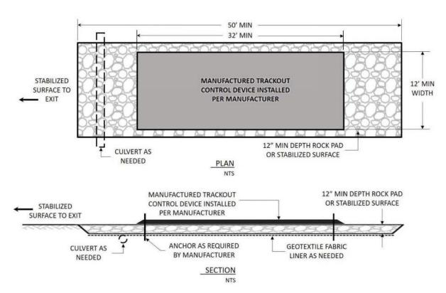
Figure 3: Example manufactured trackout control device detail.
