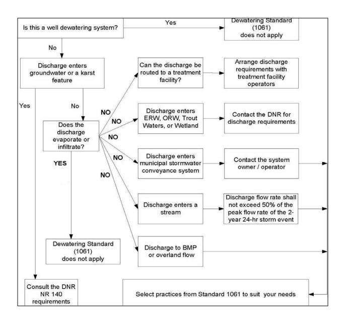
If the dewatering effluent is discolored, has an order, an oily sheen, or other toxins are present notify the DNR immediately
