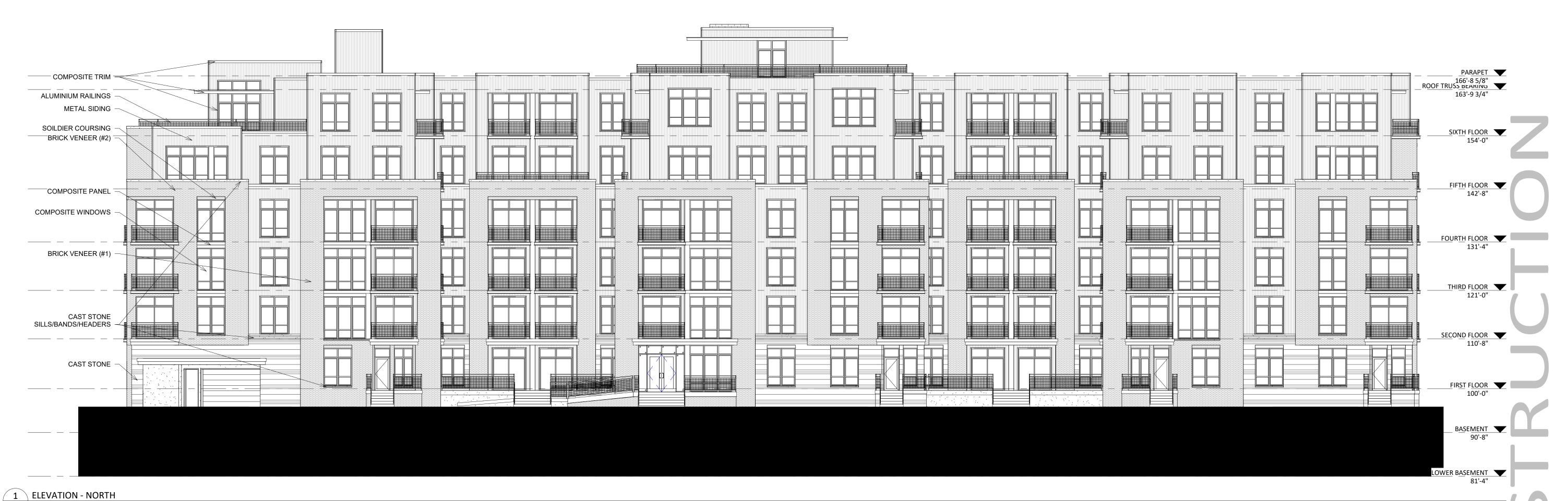
COMPOSITE TRIM PARAPET V 166'-8 5/8" ROOF TRUSS BEAKING 163'-9 3/4" METAL SIDING SOILDIER COURSING BRICK VENEER (#2) SIXTH FLOOR 154'-0" **ALUMINIUM RAILINGS** COMPOSITE PANEL FIFTH FLOOR 142'-8" COMPOSITE WINDOWS BRICK VENEER (#1) FOURTH FLOOR 131'-4" THIRD FLOOR 121'-0" CAST STONE SILLS/BANDS/HEADERS SECOND FLOOR 110'-8" CAST STONE FIRST FLOOR 100'-0" BASEMENT \
