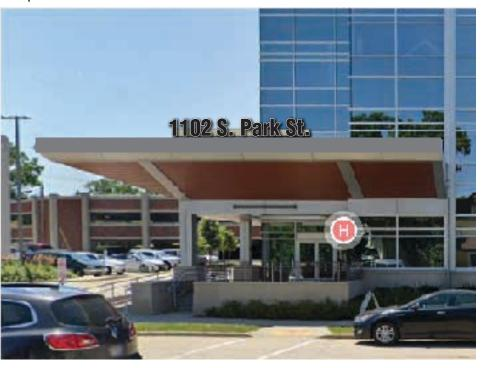
Remove 2ct existing address signs from current locations and install 1ct sign at the above proposed location.
