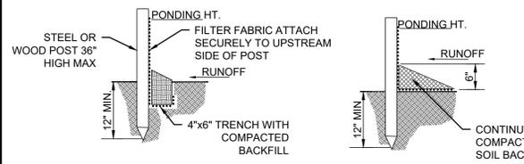
**STANDARD DETAIL TRENCH WITH NATIVE BACKFILL**
