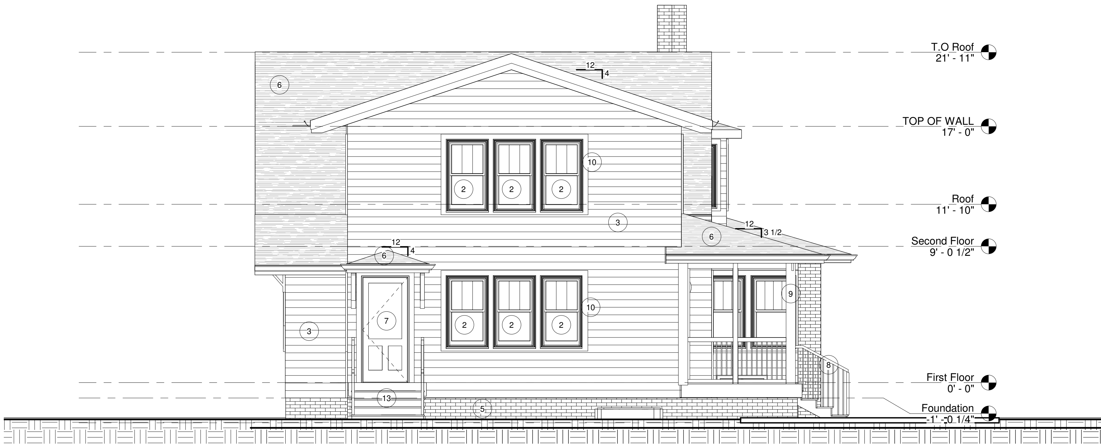
① NORTH EXTERIOR ELEVATION 1/4" = 1'-0"
