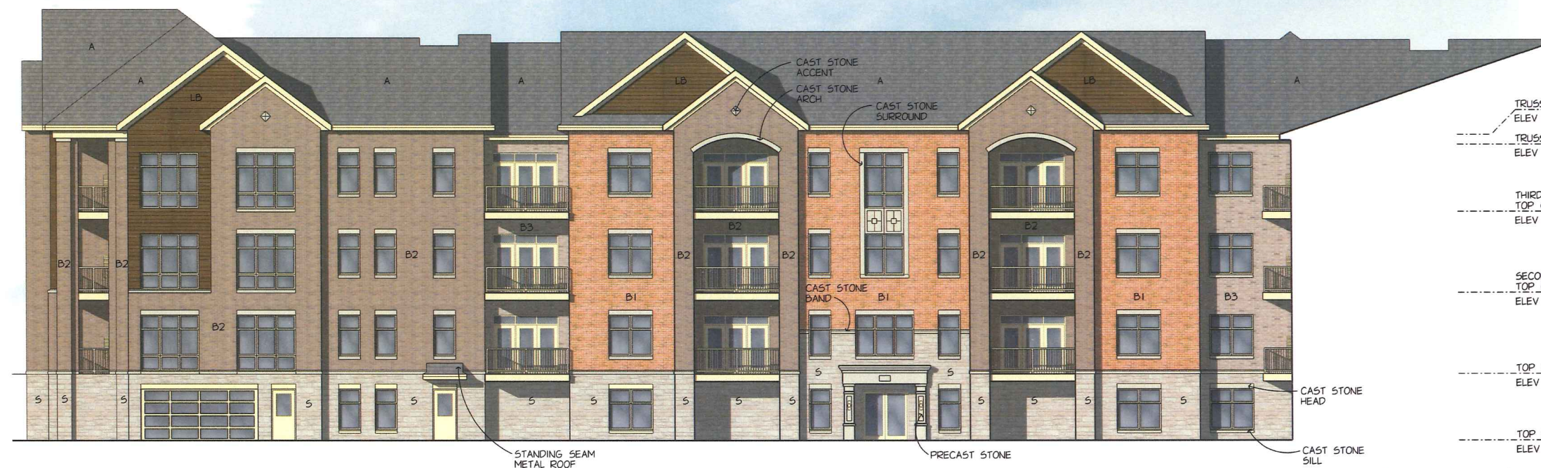
NORTH COURTYARD ELEVATION
