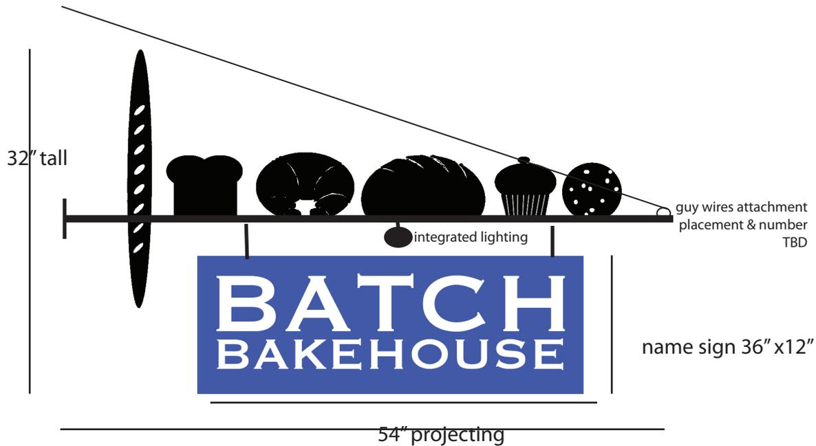
2x2 inch tubular steel welded to a heavy duty mounting plate custom universal straight arm bracket with 6 steel waterjet cut 1/4" thick bread shapes welded to top of main arm (french bread to be welded to top & bottom). Mounting bracket 6x6" with 4 - 3/8" thru holes for mounting. Color/Finish: textured black powder coat. Two 1.5" OD steel bracket rings mounted to bottom of arm for hanging name sign. 2 Guy wire rings for added support.
