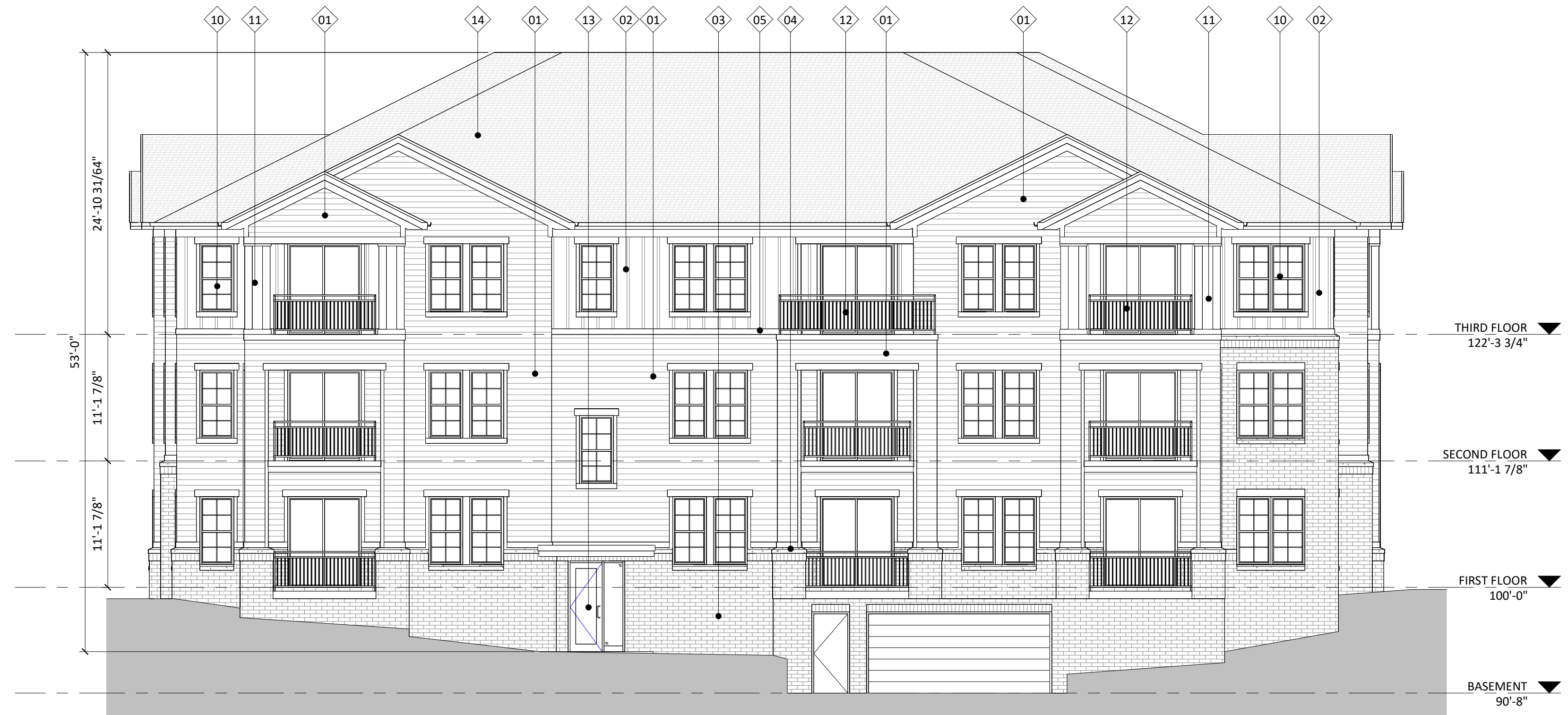
1 ELEVATION - NORTH A-2.2 1/8" = 1'-0"
