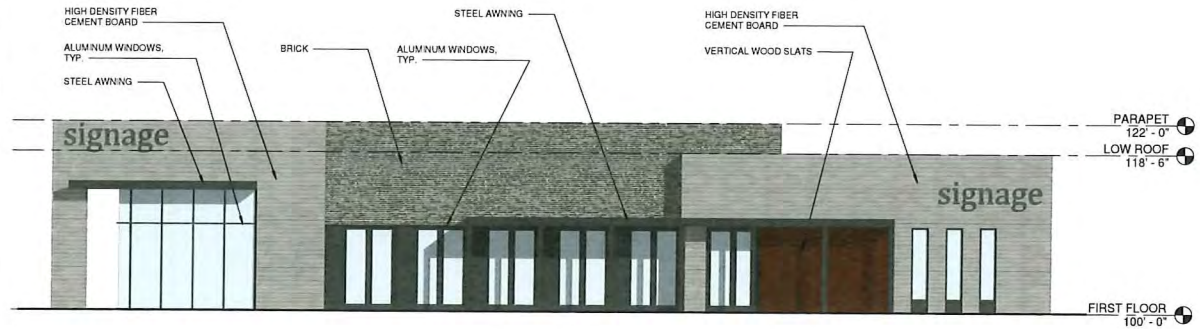
6 BUILDING D - EAST ELEVATION A220 1/8" = 1'-0"
