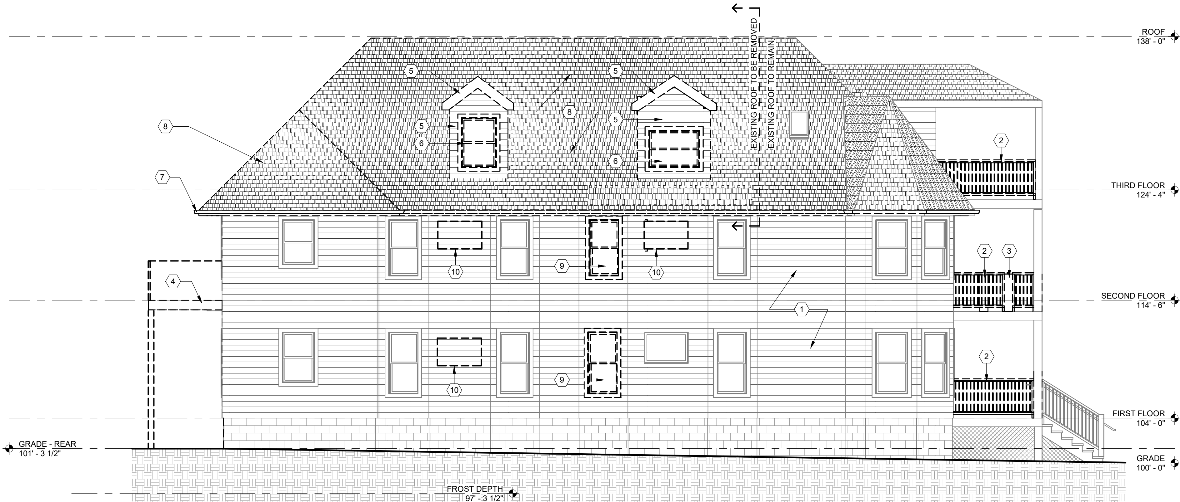
1 EAST ELEVATION - DEMOLITION 3/16" = 1'-0"
