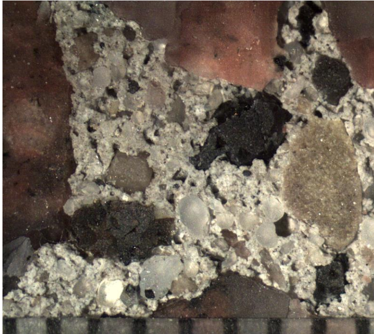
Figure 8. Photomicrograph showing an area of highly porous, very soft and chalky cement paste that has a high water-to-cement ratio (estimated to be in excess of 0.65). These soft areas comprise over 50% of the core area and are not considered resistant to freezing and thawing service conditions. Scale is in millimeters.
