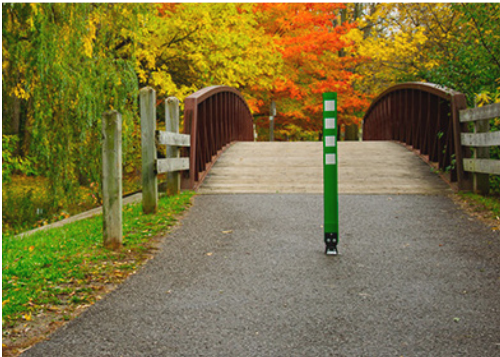
Flexible delineators at surface change/ intersections
