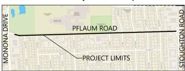
Sanitary Sewer: The existing sanitary main will be replaced along Pflaum Road. Sanitary laterals will be replaced from the new main to the property line (sanitary laterals assessable). In limited cases where the existing lateral is cast iron, appears to be in good condition upon inspection, and runs under a tree, the lateral will only be replaced to the back of curb. In those cases, the owner will not be assessed for the additional footage of replacement
