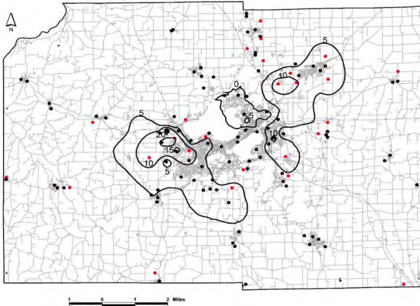
Figure 1.5. Simulated Drawdown at the Water Table, 2000-2030. Contours represent water level declines in feet.
