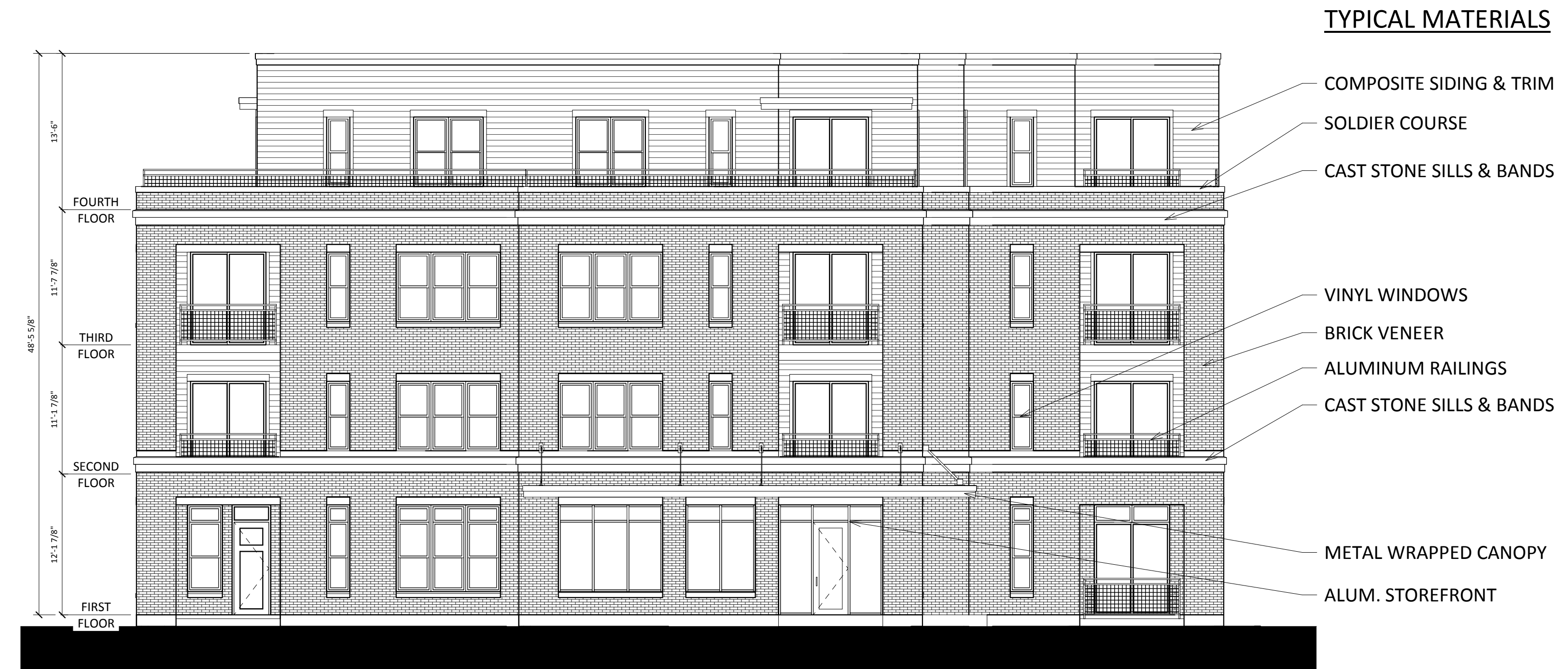
2 A-2.1 SOUTHEAST ELEVATION - ALONG E. WASH 1/8" = 1'-0"
