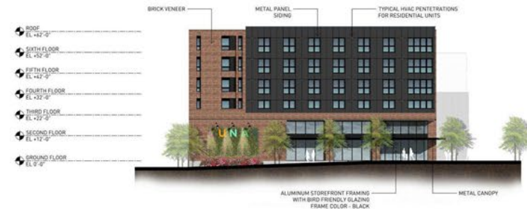
EAST ELEVATION SCALE = 1" = 20'-0"
