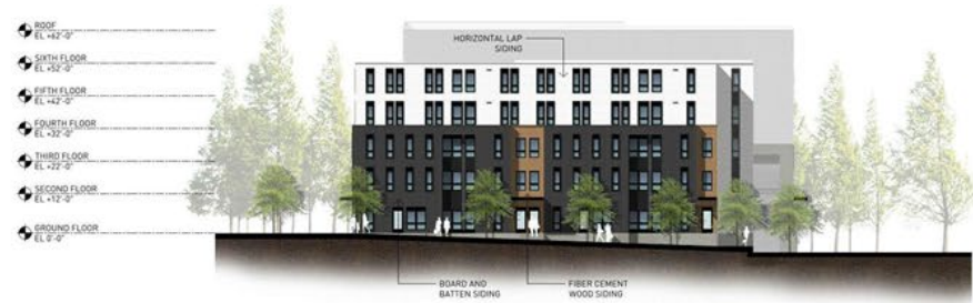
WEST ELEVATION SCALE = 1" = 20'-0"
