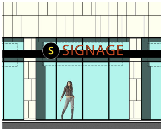
Type 8-1B: Individual letters, with individual logo Individual, internally LED-lit letters, with individual internally LED-lit logo: Logo must be formed to logo’s specific shape. Letters and logo must have metal sides and back with the same finish and must have a minimum depth of 6”.
