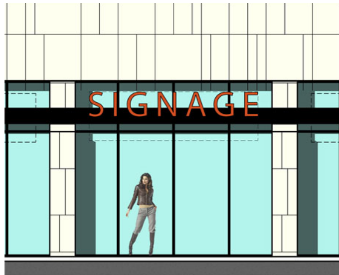
Type 8-1A: Individual letters, no logo Individual, internally LED-lit letters, no logo: Letters must have metal sides and back with the same finish and must have a minimum depth of 6”.
