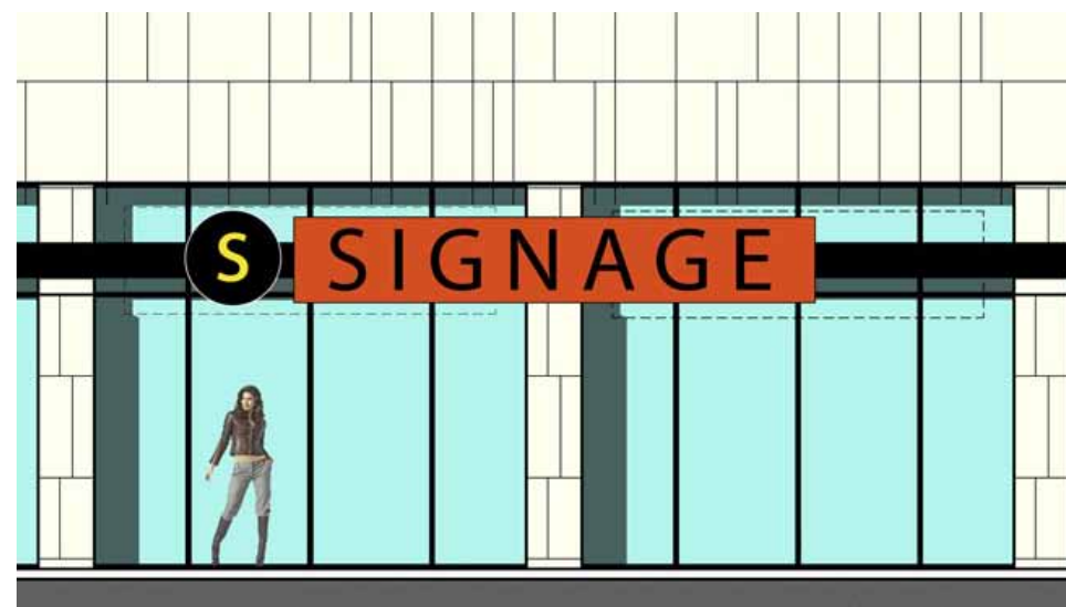
Type 8-2C: Multiple box signs Multiple box signs: Two internally fluorescent or LED-lit, metal-clad boxes (all sides). One with die cut letters and second with logo die cut to logo’s specific shape. Shape of boxes may be rectangular, but more unique shapes are encouraged. Sign must appear monolithic and have the same finish on the front, sides, and back. Boxes must have a minimum depth of 6”.
