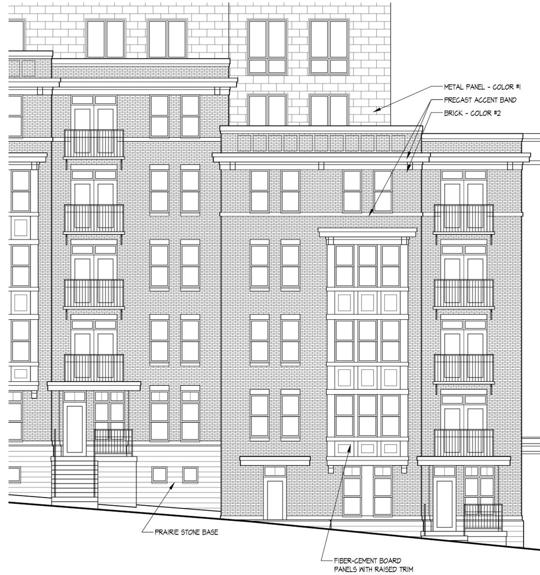
1 PARTIAL NORTHEAST DETAILED ELEVATION
