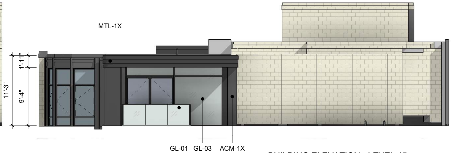
BUILDING ELEVATION - LEVEL 15 SOUTH - CAPITOL SIDE 1/8" = 1'-0"
