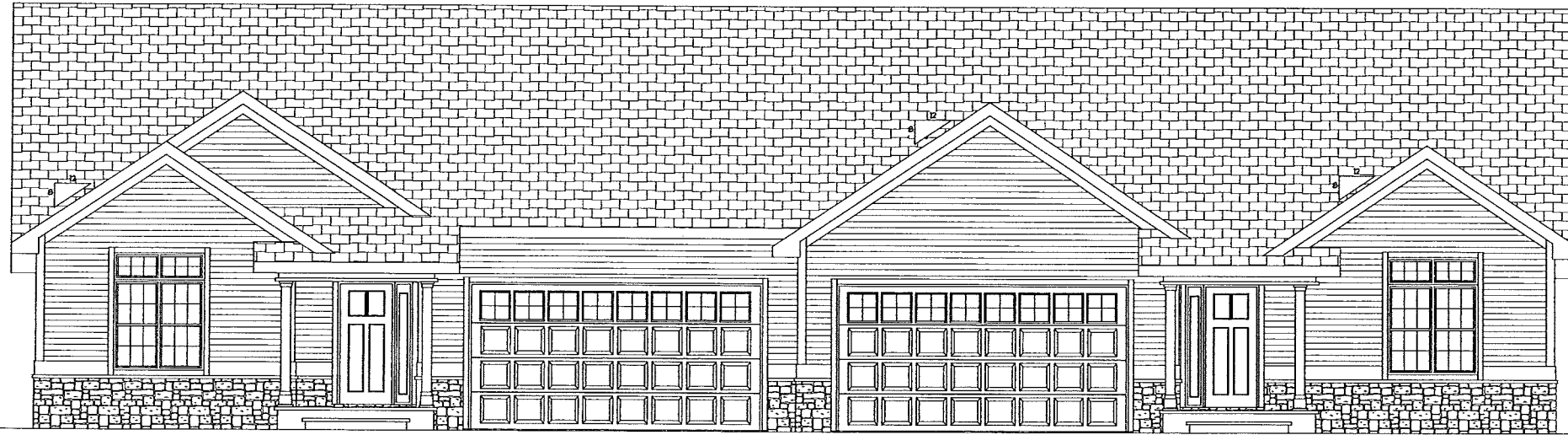
FRONT ELEVATION SCALE: 1/4" = 1'-0"
