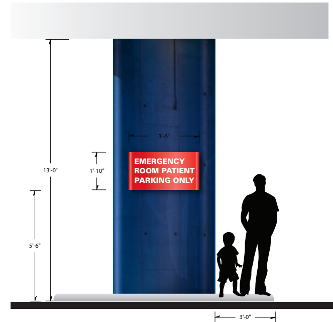
Signs on east and west sides of outside ER columns and on internal ER parking ramp areas
