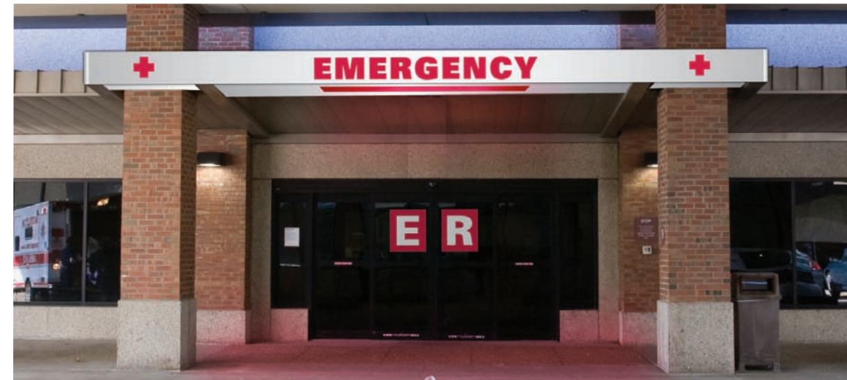
4 Emergency Entrance Marker, Under Canopy Internally Illuminated Aluminum Sign Cabinet 25'6" L x 14" H x 0'-4" D overall 25.5 sq ft signable area
